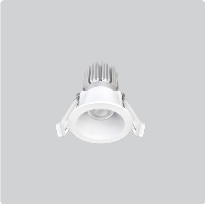
R729 Mini Dimensions D70 x H91mm Cut Out Ø57mm Watts Selectable 5.3W-8.5W Lumens <700lm Beam 45°
