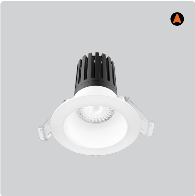
R730 Standard Dimensions D93 x H105mm Cut Out Ø 72-82mm Watts 9.5W Lumens <950lm Beam 50°
