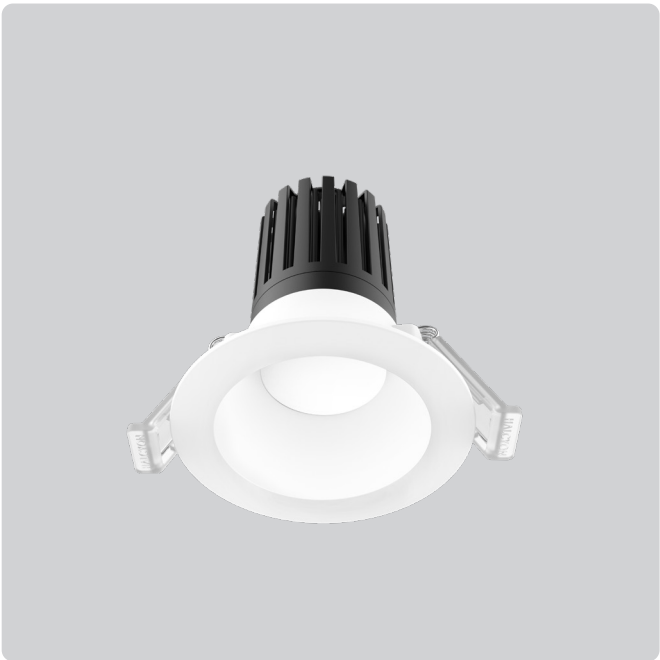
R731 Standard Wide Beam Dimensions D93 x H105mm Cut Out Ø 72-82mm Watts 9.5W Lumens <930lm Beam 90°
